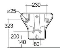
Dimensions: All dimensions in mm tolerance  $\pm 5\%$  for below 200mm and  $\pm 3\%$  for above 200mm.
