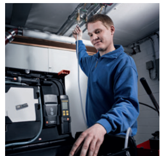
Drinking and waste water test with high-pressure probe up to 25 bar
